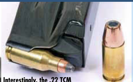
Interestingly, the .22 TCM (based on the .223 case) and 9mm both use the same magazine (18 rounds for the .22 and 17 for the 9mm).
